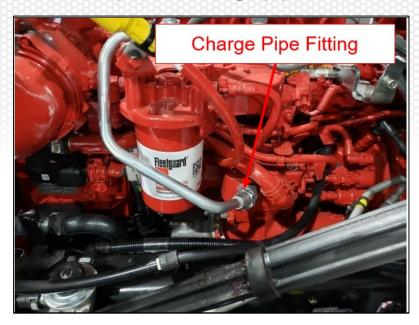
**4.** Using a 30mm crows foot wrench, tighten the flare nut to the specified torque.
