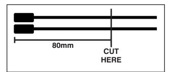
• Strip 10mm of insulation from the ends of both wires making sure that both wires are the same length when done.
