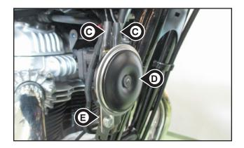
• Cut each lead wire 80mm from the end of the lead connector.
