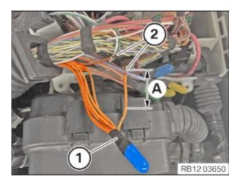
Repair Instruction 00 72 067 "Retrofitting component protection and checking function of angle fitting" indicates the splice cap is blue, this is not the actual color of the splice cap.
