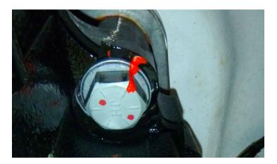
6. The following photograph shows an <u>example of a bad torque stripe</u>. Notice the torque stripes are broken due to rotation of the bolt.
