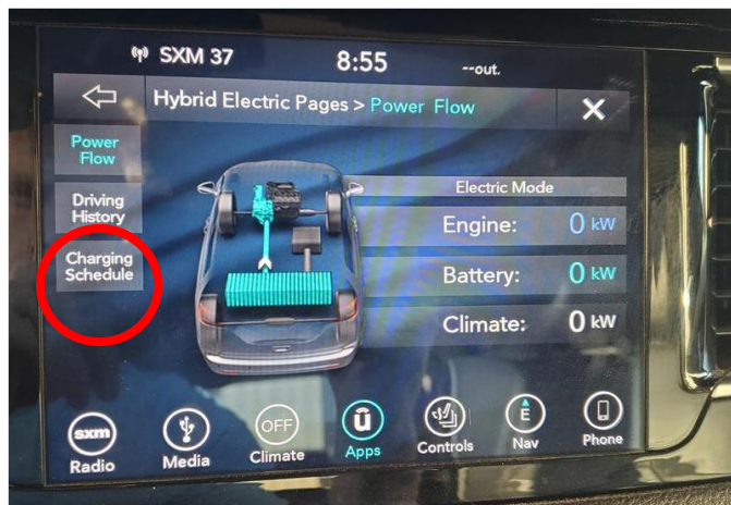
Figure 2 – Charging Schedule Display
