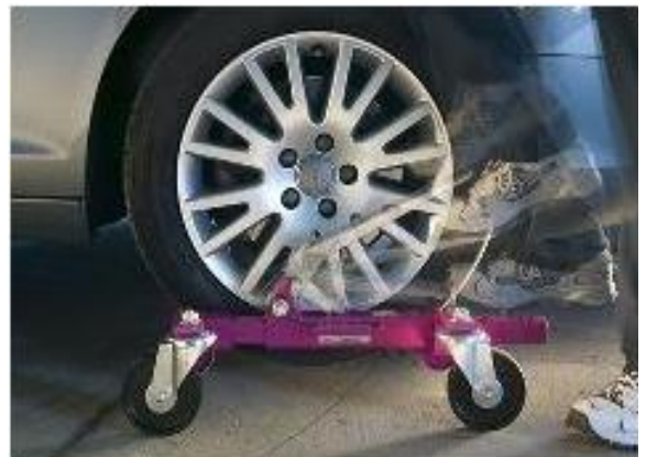
Figure 5 – Wheel Jack Dolly Installed
