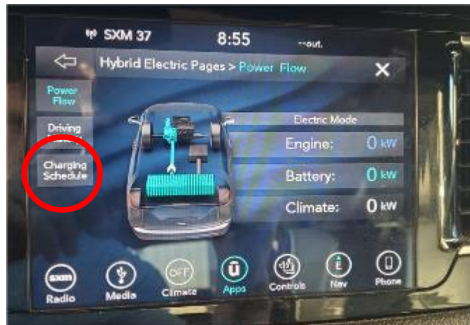
Figure 2 – Charging Schedule Display
