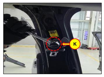
TSB #: 22-01-026H Page 5 of 7 13. Loosen the mounting bolts (L) and (M) and remove the front seat belt pretensioner.
