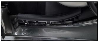
8. Move the front seat belt lower anchor cover (G) upward.
