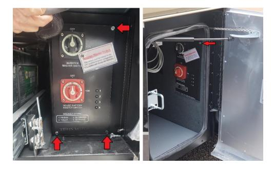
4. Remove the DCD panel, and locate the buss bar between the inverter stud and the 400A Zcase fuse.
