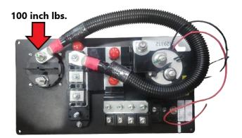
7. Loop the harness around behind the board, and connect the other end of the cable to the stud for the 400A Zcase fuse. This will require using the torque wrench set on 100 in lbs.
