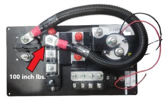
8. Install the 5129401 CVR STUD RBBR RED on the studs. This will provide protection for the added cable
