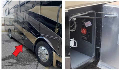
*3.* Using the 5/8" bit and the drill, remove the screws holding the DCD board in place. (The DCD board mounts in a black panel that has a flange which is held in place.
