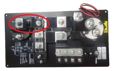
5. Using the wrench, remove the nuts from the studs, and remove the buss bar.
