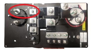
6. Using the cable provided, connect one end of the cable to the stud for the inverter switch. This will require using the torque wrench set on 100 in lbs.
