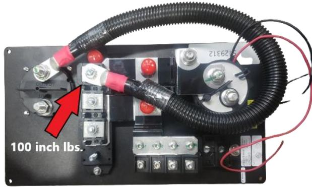
11. Install the 5129401 CVR STUD RBBR RED on the studs. This will provide protection for the added cable
