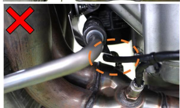
8. Start the engine and check for leaks from the newly installed oil cooler outlet pipe.
