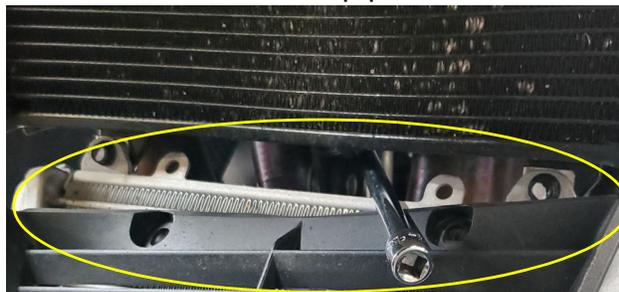
4. Install the new oil cooler outlet pipe to the engine. Reinstall the oil pipe plate and bolt.
