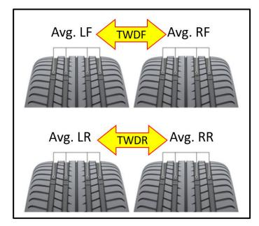
Calculate tread wear difference (TWDx) on each axle:
