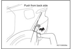
Note: To protect the rear bumper assembly from breakage, push the area around the claws from the back side by inserting your hand from the gap between the rear bumper assembly and vehicle body.
