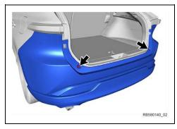
e. Install the 2 rear bumper stoppers (screw and grommet).
