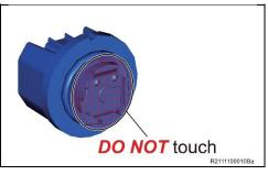
DO NOT touch the printed circuit board of the new rear turn signal light LED, since static electricity may damage the LED.
