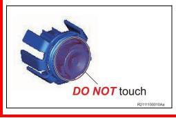
DO NOT touch the printed circuit board of the removed back-up light LED, since static electricity may damage the LED.
