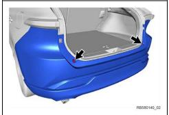
d. Remove the 2 rear bumper upper stoppers (screw and grommet).
