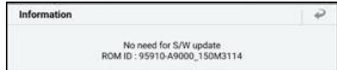
**Note:** This pop-up notice may display if the ACU does not need or match the selected update. Please, check the ACU parts number and select correct match by referring the Manual upgrade list. If the pop-up notice continues to display, even though ACU part is correctly matched to the Manual upgrade list in this bulletin, then the ACU part will not require the upgrade event.
