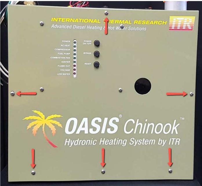
Remove these screws to gain access to the inside of the heater.
