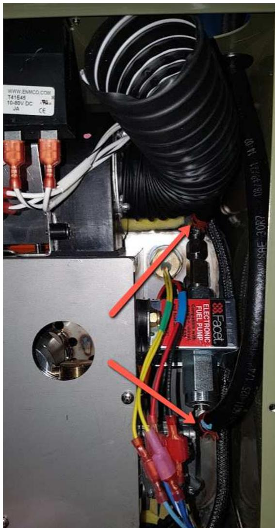
1. Using angled needle nose pliers, move the clamp off both fuel pump fittings and pull out both generic hoses, using a rag to catch any fuel that spills.
