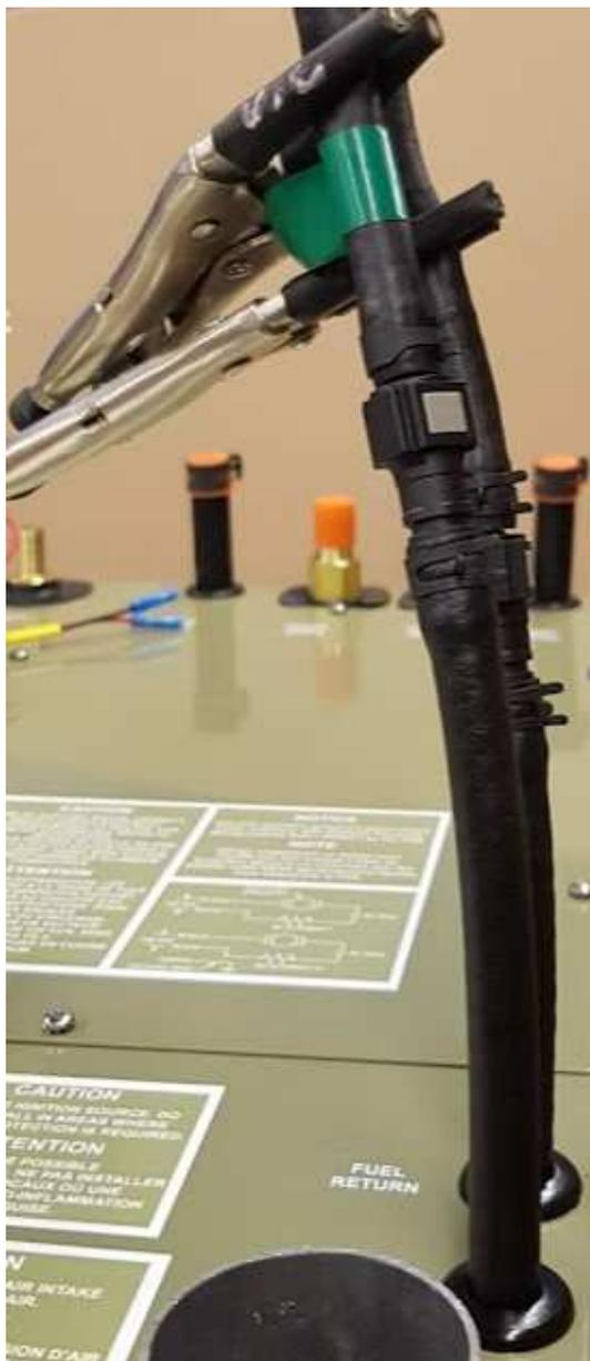
1. Mark the fuel inlet line and clamp off the fuel inlet and return lines above the quick connects.
