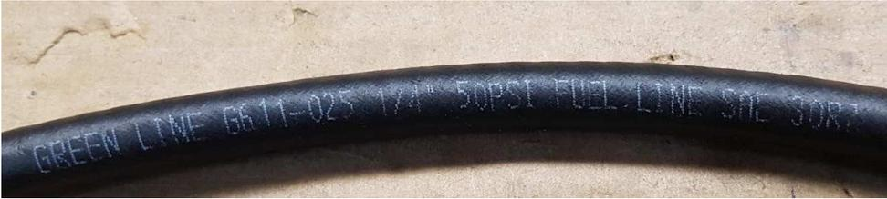
The above fuel line is the correct type. It has "FUEL LINE SAE30R7" marked on it. The incorrect hose can be identified by either marking of "VALUFLEX/GS" or by what appear to be holes in the hose as shown below.
