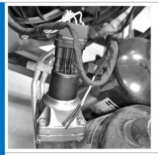
Locate LIV wires at CSMV and cut cable tie securing to harness.
