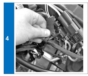
Apply tape (A1) to harness to secure LIV harness leg/wires to the harness main .
