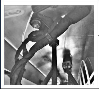
Bundle harness as shown and secure harness with cable tie (J) to cable tie base.
