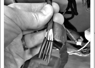
Wrap wire ends together with tape (A1) . Continue wrapping tape to end to cover heat shrink.
