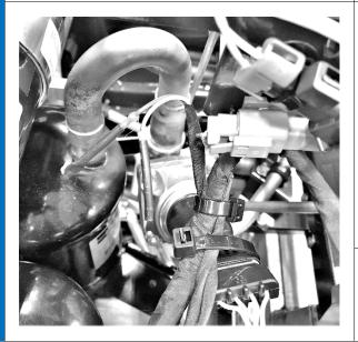
Install heat shrink caps (K) on both of the wires and use heat gun to seal.
