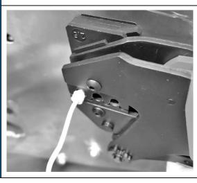
Crimp terminals and seals to the wire. Use the appropriate die position for the size terminal being crimped.
