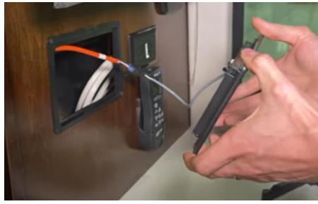
Reinstall Touch Screen in its mount
