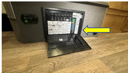
Open Fuse Panel and Locate Awning Fuse
