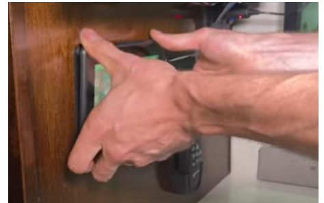
Reinstall Touch Screen – push firmly in place
