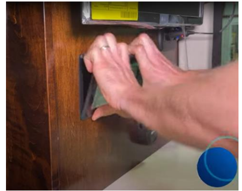
Remove Touch Screen from wall bracket
