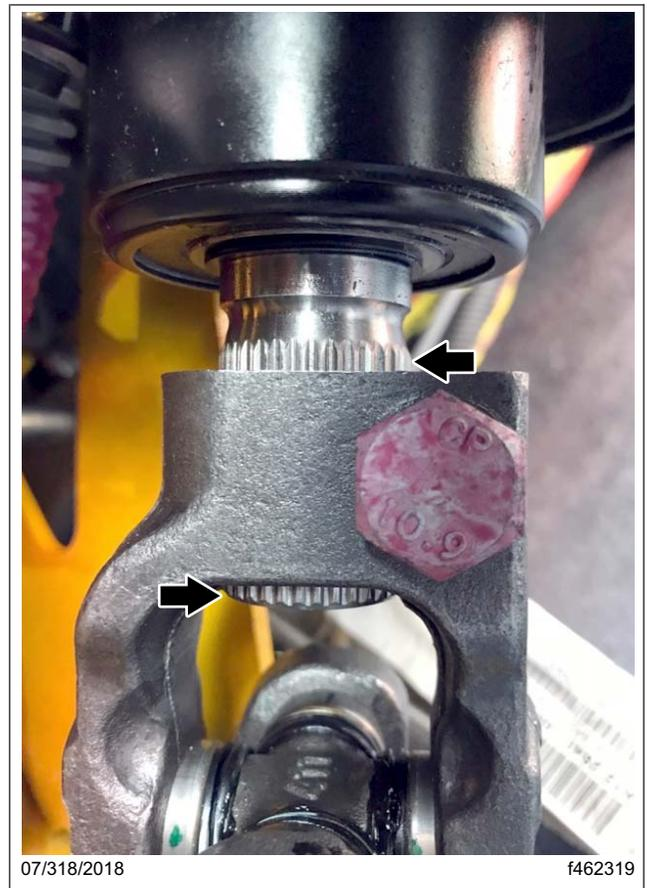
**Fig. 2, Steering Shaft Splines**
