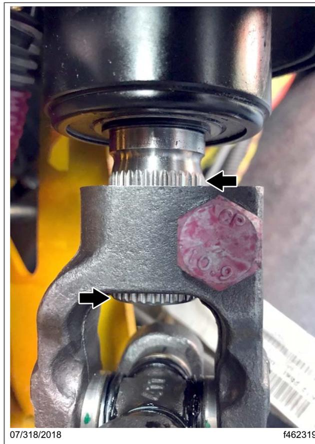
**Fig. 2, Steering Shaft Splines**
