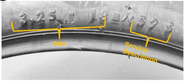
According to the example: Size 3.25-18, Service Description (Load Index + Speed Symbol) 59S
