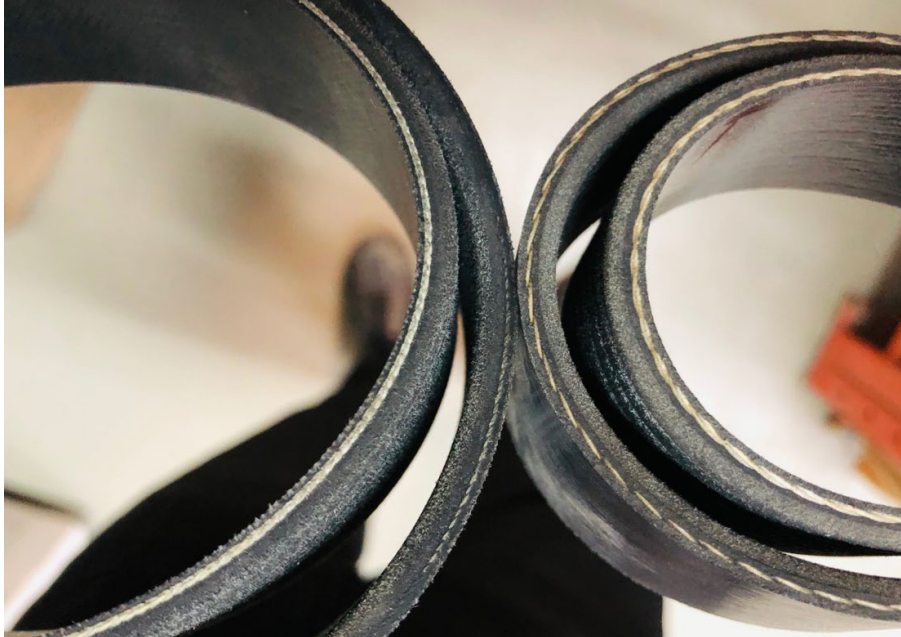
Defective Aramid cord reinforced belt (left) vs New polyester cord belt (right) – Note the different cord arrangement between the two belt types.
