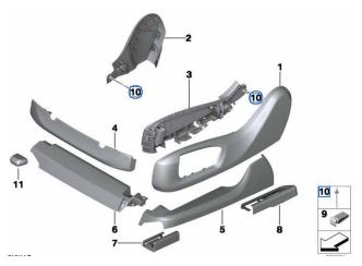
Seat plastic covers are held by blind rivets which may have to be replaced for access (7042164 blind rivet).
