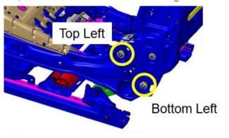
Check both outer seat backrest retainer screws. If the screw is found loose then it must be replaced (9908419 Countersunk screw - M10x16).
