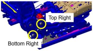
Check both inner seat backrest retainer screws. If the screw is found loose then it must be replaced (9908419 Countersunk screw - M10x16).
