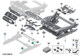
Seat rail mounting screws must be replaced once seat has been removed (9321690 Fillister head screw - Qty 4).
