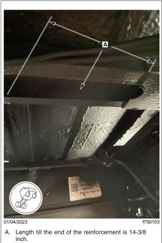
Fig. 3, Installing the Joist Reinforcement
