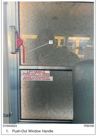
Fig. 5, Inspecting the Push-Out Window Handle Clearance
