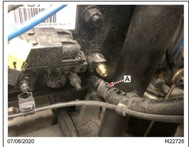
A. Remove the threaded air line that connects the modulator valve to the brake chamber.
