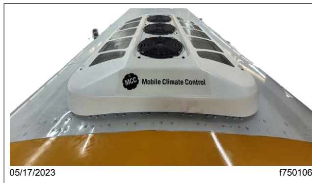
Fig. 4, Vehicle Equipped with Factory-Installed Roof-Top A/C Unit
