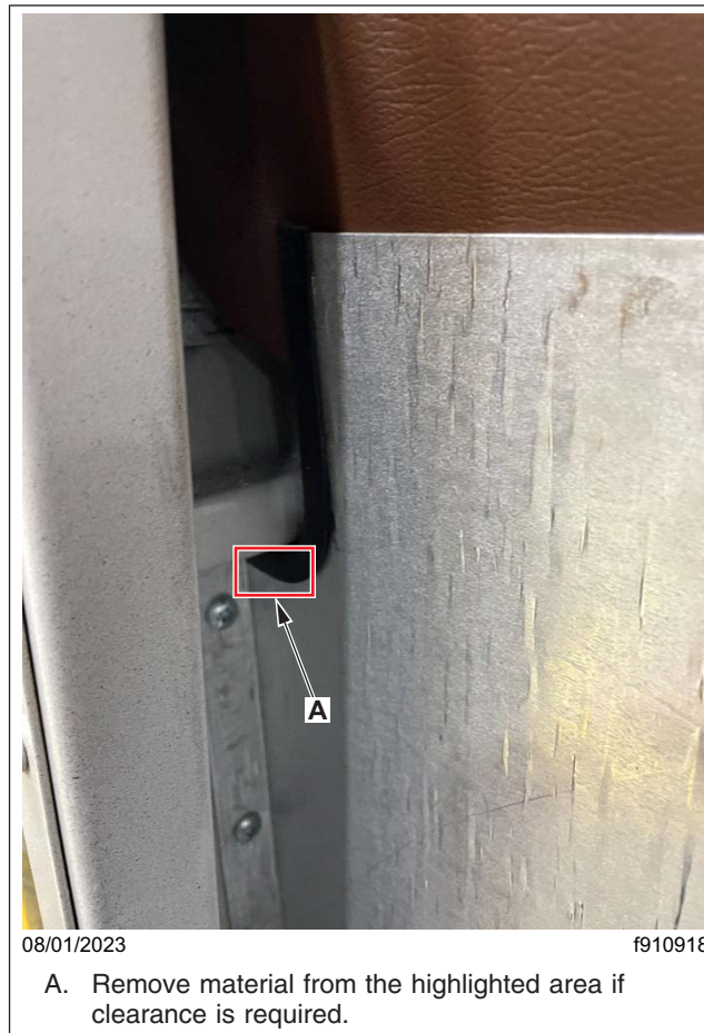
Fig. 10, Trimming the Kick Panel to Clear the Seat Rail
