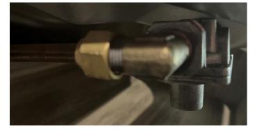
Use gas leak solution on the connection and also do a LP drop pressure test.
