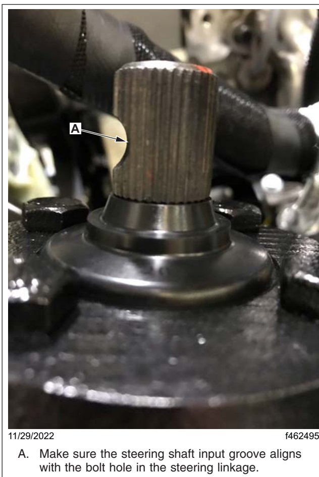
Fig. 10, Steering Linkage Installation
