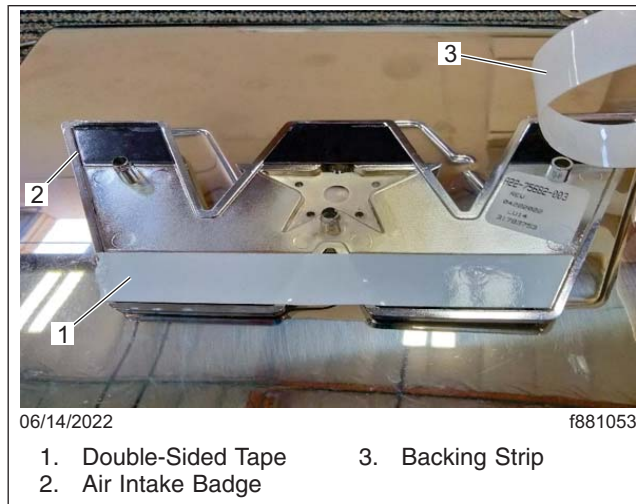
Fig. 10, Backing Strip Removal from the Double-Sided Tape
