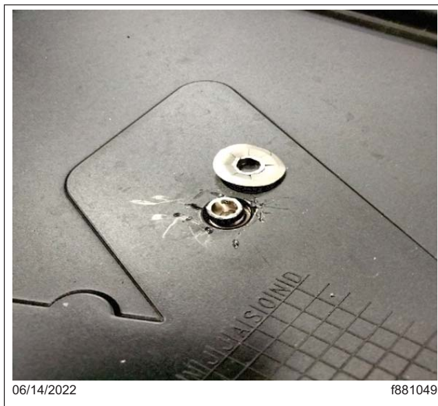
Fig. 6, Retaining Washer Removal
