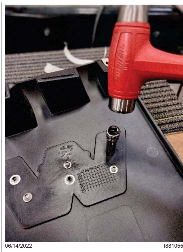
Fig. 12, Retaining Washer Installation
