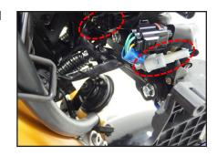
4. Disconnect the gray 2-pin connector of the grip warmer and the white 6-pin/white 3-pin connectors for the switches.
