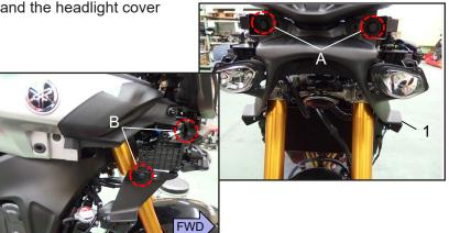
5. Remove bolts "a" and collar "b," and fuel tank cover assembly (right) "1."
