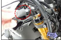
3. Disconnect the white 2-pin connector (electronic suspension [right]) and the black 6-pin connector of the handlebar switches.
