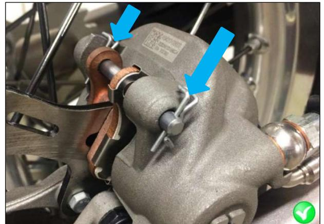
Fig 3. – Correct rear brake mounting
