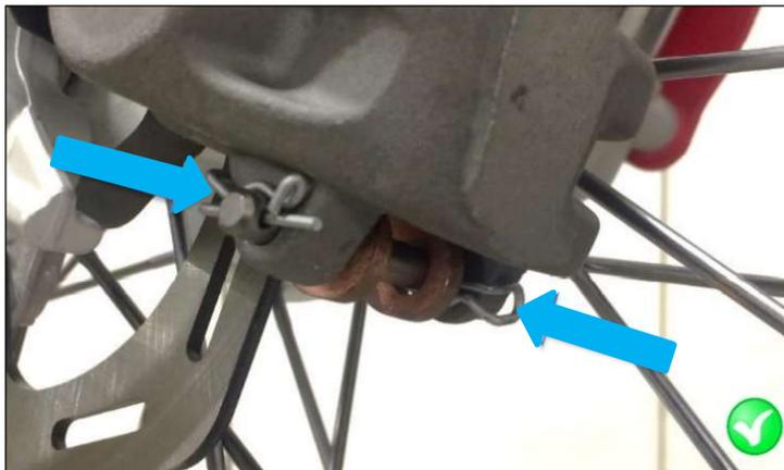
Fig 2. – Correct front brake mounting
