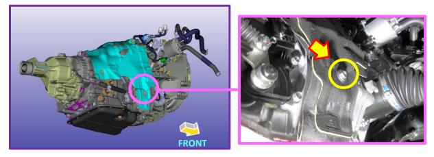
**STEP 8B: CAREFULLY** lift the insulation only as far as necessary to expose the plug as shown below.
