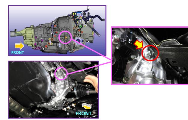
STEP 8C: Install and align the specialty plug / holder (18361AA090) as shown below.
