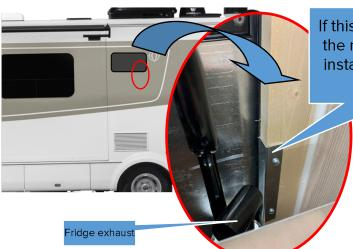
If this deflector is present, the new deflector will be installed over top of it to extend it.
