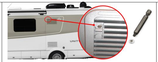
Remove the #8 screw from the top corner of the fridge vent using a #2 Robertson bit put aside for later.
