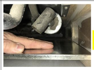
Press the heat shield in place to ensure that the silicone is making good contact with the baffle.
