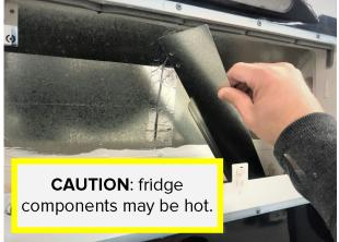
Insert the heat deflector through the top vent with the two holes at the top and with the silicone surface against the wooden frame.
