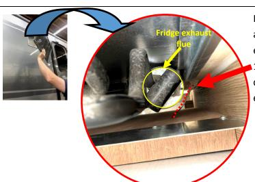
Look down the vent and locate the entry assist handle 12V wire routed close to the Fridge exhaust flue.
