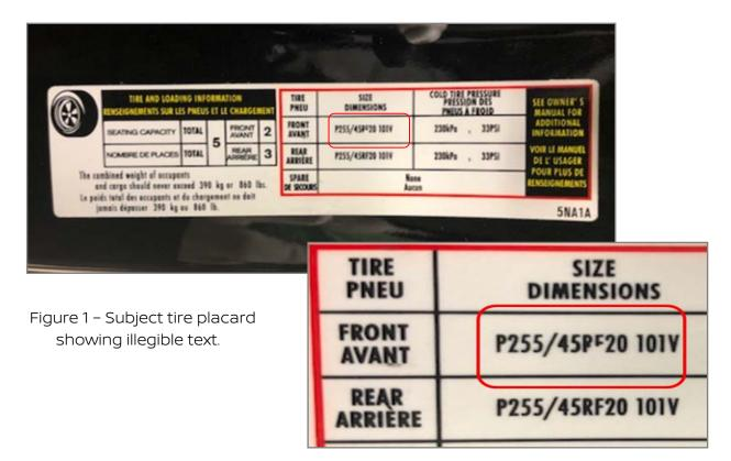
Out of 17,450 total placards inspected, 82 placards were found to have partially illegible black-text characters, resulting in an incident rate of 0.47%.
