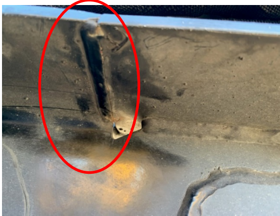
Photo 5 Crack example: frame horizontal top
