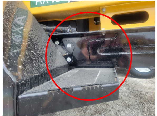
Photo 6 Crack example: frame vertical center
