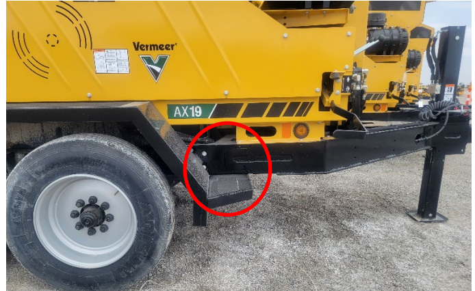
Photo 4 Potential crack location – right side
