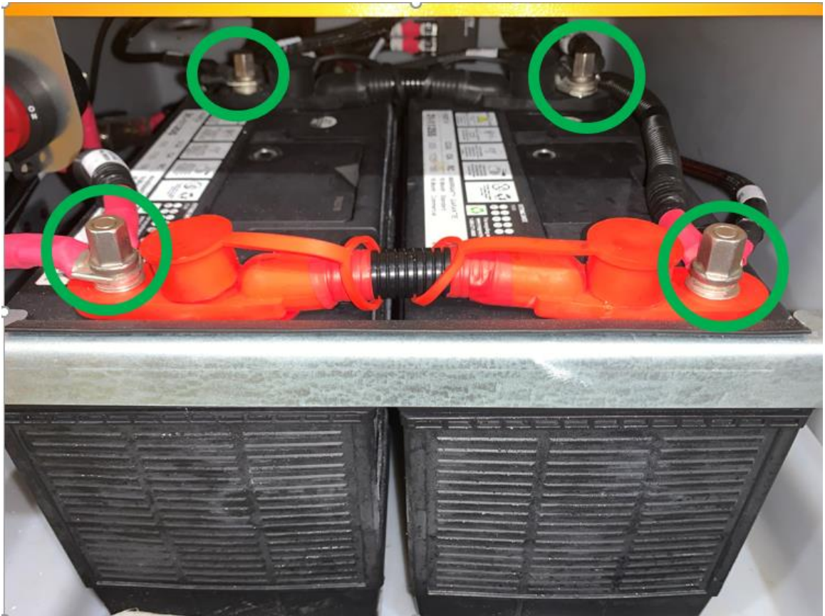
Figure 10: Battery cable lugs (195 in-lbs)
