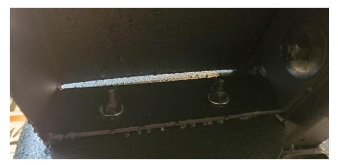
Loosen the 4 fender bolts attaching the fender to the front and rear box. These will only need slightly loosened as the intent is to slide the fender inward to create more room for the tire. Push the fender inward as far as it will go.
