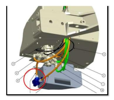
6. Avoid kinking the hoses and secure the hose bundle with cable ties.
