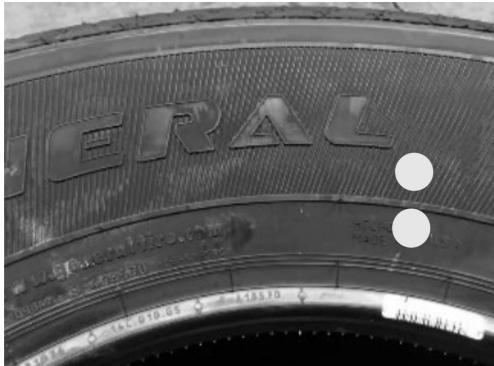
Drill two 13mm holes in the tire sidewall. Do not drill through the DOT code or bar code sticker.
