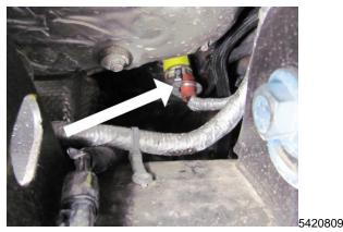
4. Looking through the area between the wheelhouse liner and the suspension, locate the engine block heater.
