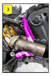
2 E. Tighten the 2 self-tapping screws (53) securing the heat guard to 1.6 Nm ± 10%.
