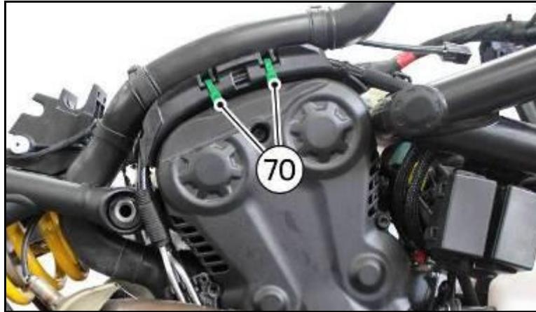
3. Remove the adhesive tape from the intake manifolds
