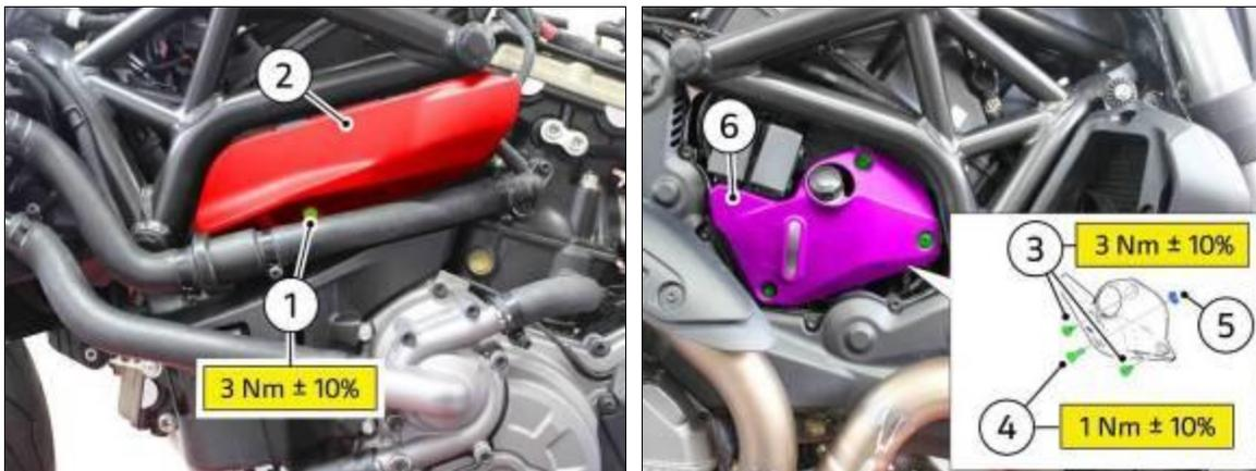
14. Fit the fuel tank (See Sec.8: "Fuel/exhaust system – Fuel tank" of the Workshop Manual)
