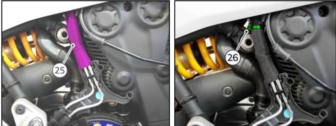
24. Position **spacers (17)** and **(23)** on ABS hose support inner side, aiming them as shown in the figure
