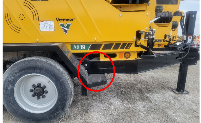
Photo 4 Potential crack location – right side
