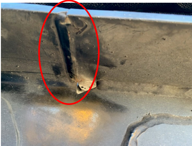
Photo 5 Crack example: frame horizontal top
