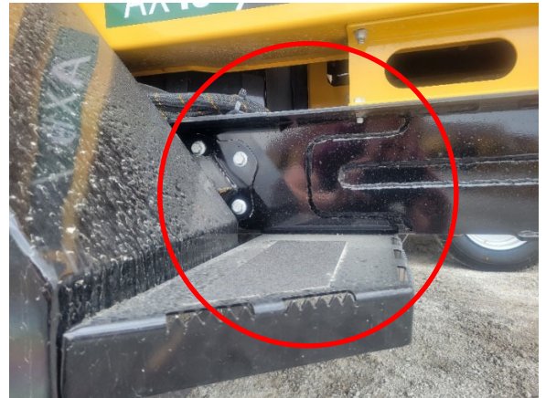
Photo 6 Crack example: frame vertical center
