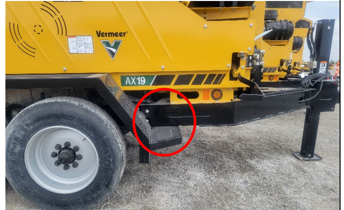
Photo 4 Potential crack location – right side
