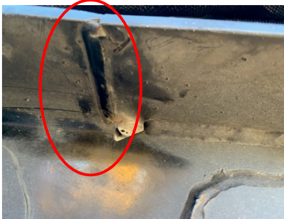
Photo 5 Crack example: frame horizontal top
