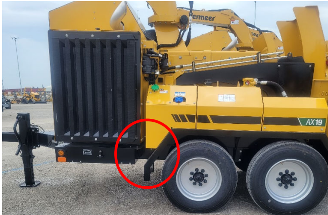
Photo 3 Potential crack location – left side (near V-cut out in frame) Engineering analysis indicates the left side may be more susceptible to crack(s) forming.
