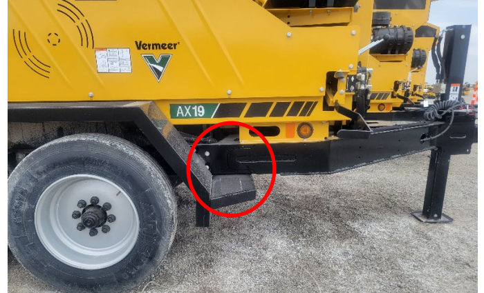
Photo 4 Potential crack location – right side
