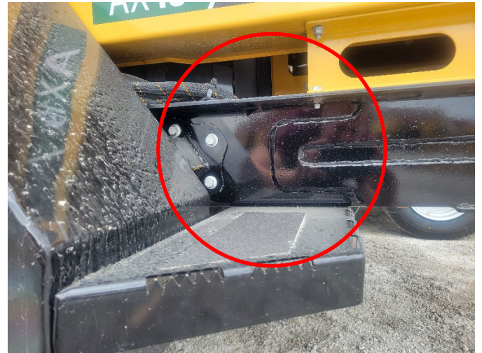
Photo 6 Crack example: frame vertical center
