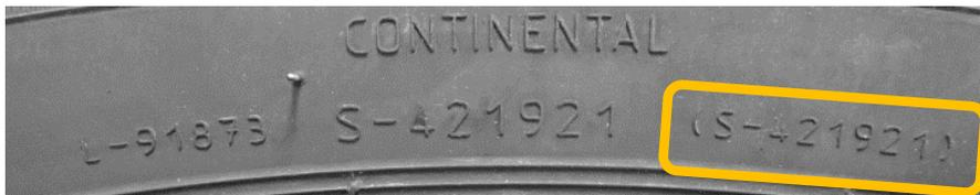
Mold number identification example: "S-" 421921 or without the "S-" like the mold number below,
