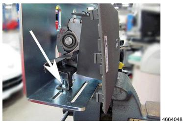
2. Using the hardware kit supplied with the module bracket, loosely mount the airbag assembly to the bracket using two nuts and bolts.
