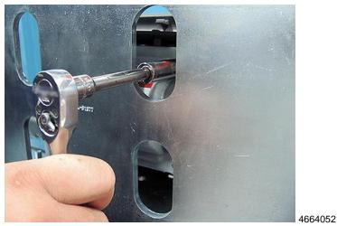
2. Use the access holes in the bracket to loosen and remove the four self-locking nuts, **do not use power tools to remove the nuts.** Discard the nuts, they will not be reused.
