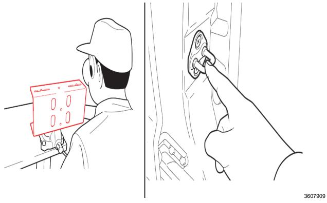
**Danger:** To avoid personal injury, *ALWAYS* keep as much of your body as possible in front of the bracket when working on the airbag assembly. Remember to periodically touch a metallic part of the vehicle or work bench to discharge static electricity in the body. DO NOT use power tools when performing the inflator removal/reinstallation steps.
