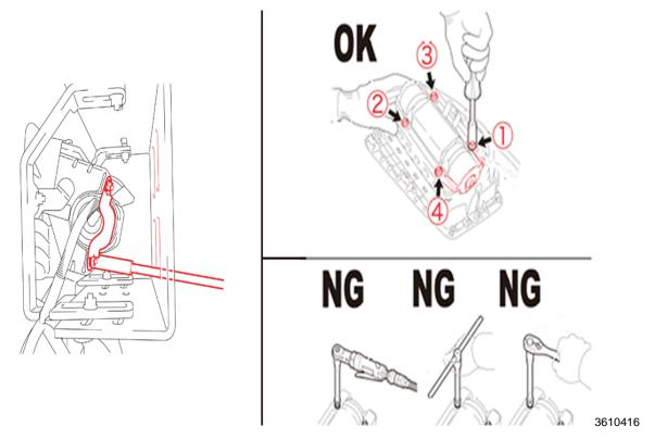
14. Tighten four (4) *NEW* plate nuts evenly in several increments in the order shown in the illustration using a 10-mm socket driver while pushing the inflator. You will encounter some resistance during tightening because these nuts are self-locking nuts. **Torque Specification: 6.5 Nm (57.53 in-lb).**
