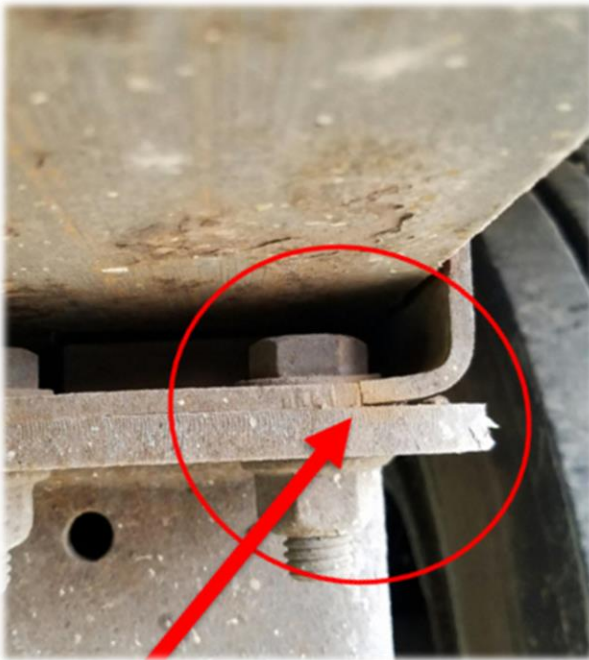
Crack near the inside bolt.
