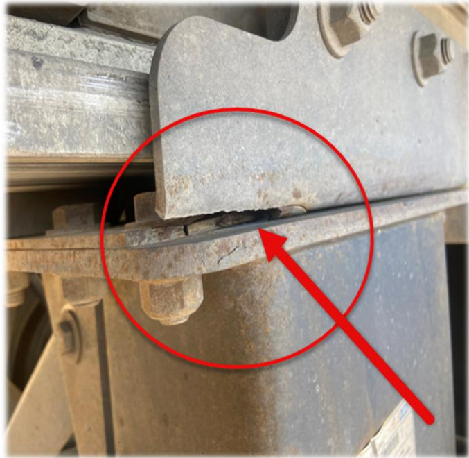
Crack on rounded edge of pan.
