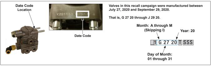
Figure 3 - SR-7 Spring Brake Modulating Valve Date Code Interpretation
