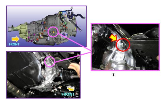
STEP 3C: Install and align the specialty plug / holder (18361AA090) as shown below.
