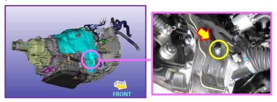
STEP 3B: CAREFULLY lift the insulation only as far as necessary to expose the plug as shown below.
