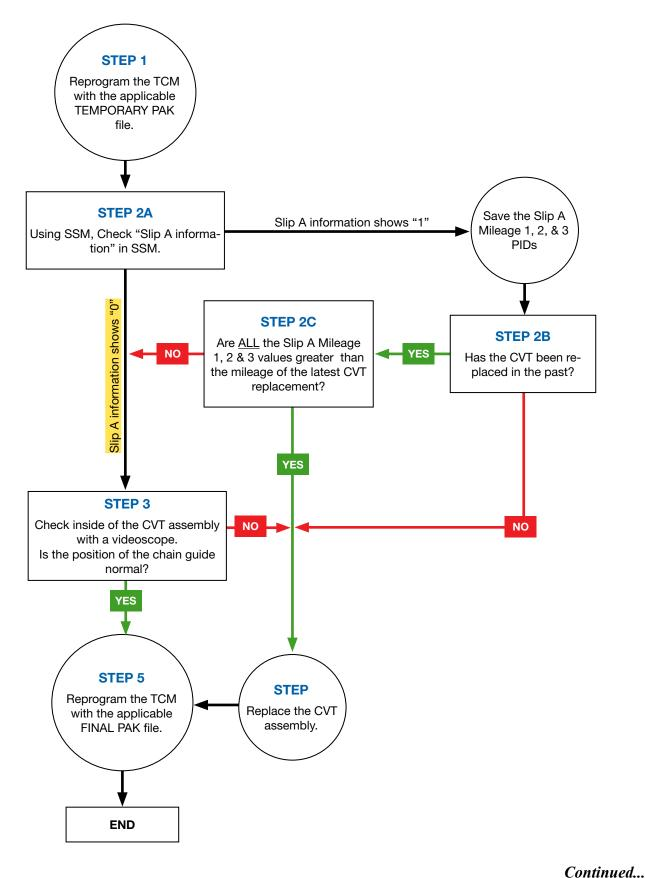
**STEP 1-A:** Perform a DTC check of the TCM and confirm there are no current faults. Any previous faults must be diagnosed, repaired, and cleared prior to reprogramming. Reprogram the Transmission TCM with the **TEMPORARY** PAK file.
